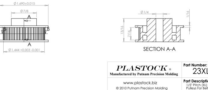
Part Description: 1/5" Pitch (XL) Timing Belt Pulleys For Belts up to 3/8" Wide
